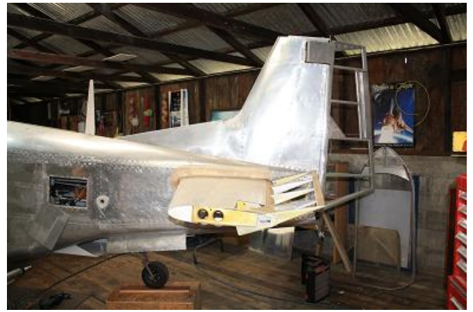
The T-51Empennage. The rudder will be fabric covered.
