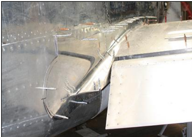
The wing fillet made on an English Wheel.
