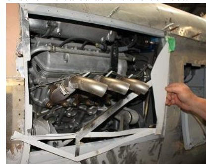
Warren holds a mockup of his new mount design. The diagonal will be a turnbuckle
