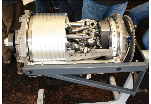
The larger Duke Engine in cutaway.
